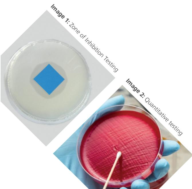
Image 1: Zone of Inhibition Testing
